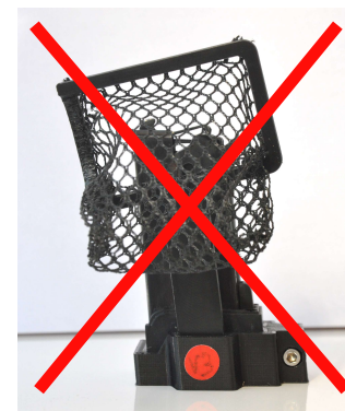
BAD POSITION ON THE MAGAZINE (REVERSED).
