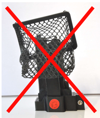
BAD POSITION ON THE MAGAZINE (REVERSED).
